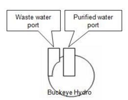
Tubing should be installed to go from the permeate port to a check valve, (with water allowed to flow only towards the ASO valve, to the LP-in port on the ASOV, to LP-out port, to DI housing (if you have one), to your final use.
