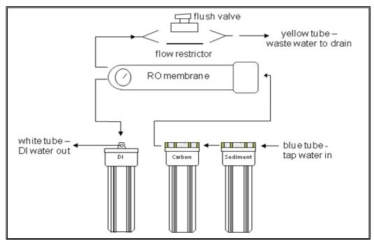
into the sediment filter "in" port, and the DI housing "out" port. Screw the DI housing back into place.
