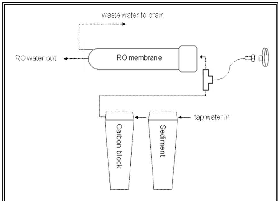
Along with water temperature, pressure is a critically important parameter in determining how well your system operates. The purpose of the pressure gauge you've purchased is to display the pressure present in the system that will affect the performance of the RO membrane. Factory specifications for Filmtec membranes call for 50 psi; specifications for residential membranes produced by other manufacturers are commonly higher (e.g., 60 or 65 psi).
