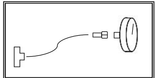
Wrap the male threads on the back of the gauge with Teflon tape. Screw the female adapter to these threads, being careful not to cross thread or over-tighten the plastic fitting.
